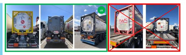
All vehicles for bulk product transport shall be equipped with 3 independent closures in series for bottom filling or discharge openings. This includes an internal valve (bottom / foot), an external valve and a final closing device.
