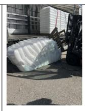
Forklifts can tip over whereby the forklift driver may be thrown out of the cabin and become fatally injured when the forklift falls onto him, **therefore**, **seat belts must be worn**.
