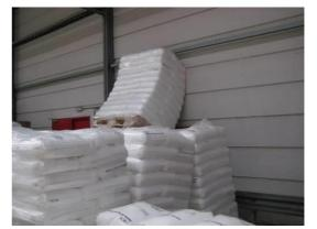
Always leave 1 meter distance between the pallets and the warehouse walls. If this aisle is used as a pedestrian walkway, do not double stack the pallets closest to the walkway.
